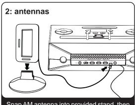
Snap AM antenna into provided stand, then plug antenna cable into socket on back of iD84. Move antenna 12" away. Extend FM antenna.
